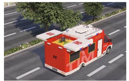
Multiple charging for drone fleet in emergency response vehicle
