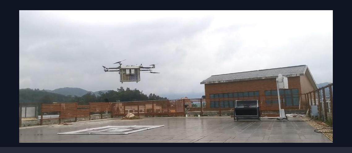
Phoenix Wings Ark 40, HEISHA D80 UAV dock, together forming the Resistance Emergency Response Network system in Dapeng.
